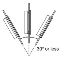
When installing the panel in a slanted position with an incline more than 30°, the ambient temperature must not exceed  $40~^{\circ}$ C ( $104~^{\circ}$ F). You may need to use forced air cooling (fan,A/C) to ensure the ambient operating temperature is  $40~^{\circ}$ C or less (104 °F or less).
